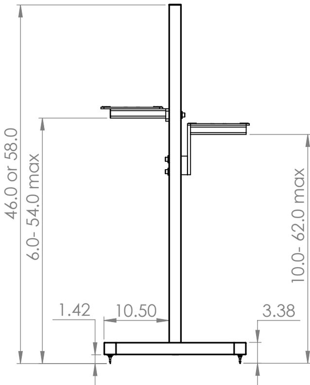
Platform can be rotated 90° so that width and depth are interchangeable
