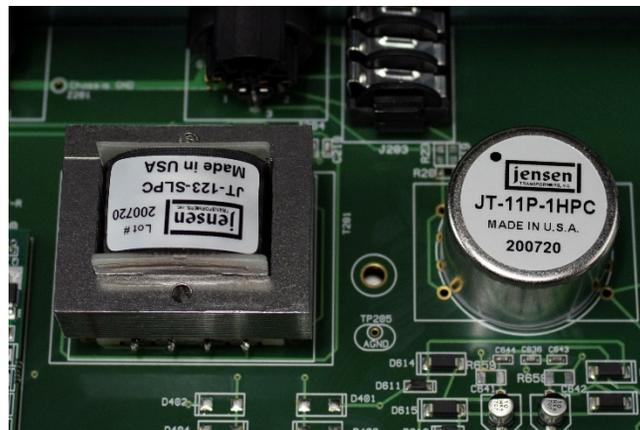
**Why it’s Different:** The Daking Comp IIT is a complex design that employs a unique method of gain reduction using a VCA like a FET. This maintains the unique Daking sound of our legacy compressors. Unlike most VCA designs, ours uses feedback gain reduction, a peak detector and an all-discrete Class A follower. The Jensen transformers add some subtle analog color.
