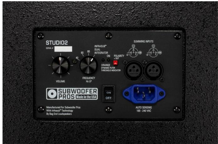
The SUBWOOFER PROS Studio Sub2-18C is a “universal” sub used for bass extension of any studio monitor. It is sealed and self-powered, offering bass extension to 16Hz. It has a compact cabinet using an 18” high excursion sub driver with an easy to use control set. It has built in Left/Right XLR summing inputs and a low pass filter at 4 different frequencies of 95Hz, 80Hz, 60Hz, and 40Hz. The different low pass frequencies make it adaptable to various size “main” speakers.
