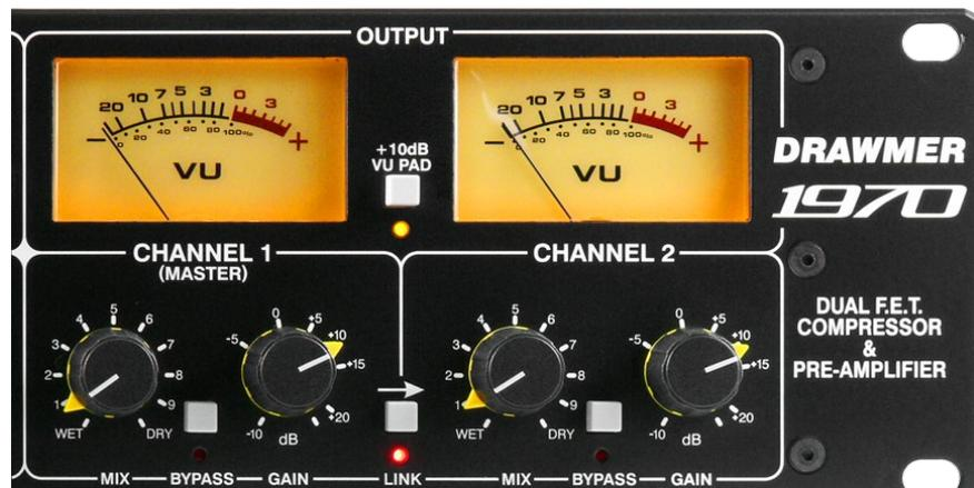
At the right side of the front panel are Gain control knobs for Ch1 and Ch2. The Gain controls have a range of -10 to +20dB and act as a fine adjust for the overall level through the 1970—whether you're using the compressor or not. With the compressor switched in, these are used to add more level to get parity—match the same approximate level as the uncompressed signal from just the pre-amp section.
