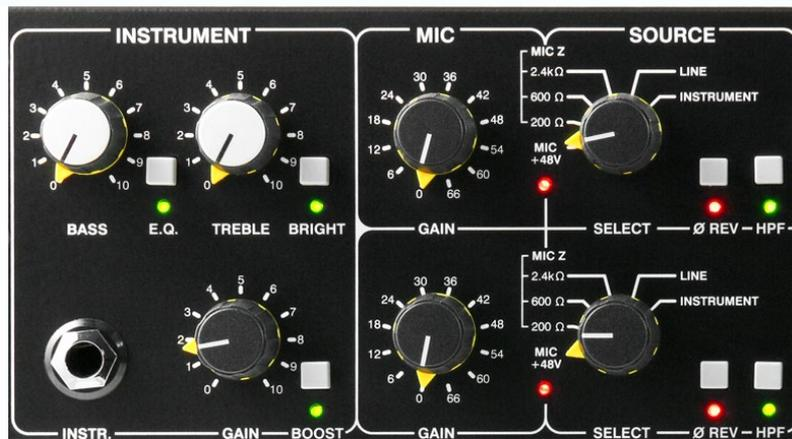
After the Source switch come separate Phase (or polarity) reverse and a 70Hz HPF or high pass filter switches. The Phase switch is when recording the same source with two mics—one coming into each channel. Normally, you should not have to use it unless one of the microphones or the connecting cables is miss-wired.
