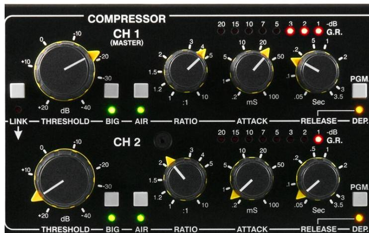
Turn the compressor Link switch off, the large Threshold control should be at full CCW at +20dB, both the Big and Air switches should be off, and make sure
