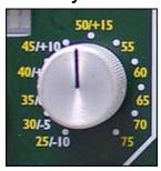
Your Mic Pre IV is equipped with rotary switches which make a click when you turn them. Switches are more reliable and have a higher tolerance than rotary potentiometers, which are the smooth turning knobs on an electric guitar or your stereo's volume knob.
