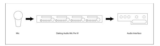
Patch from the microphone to the mic input on the MPIV using the female XLR to male XLR microphone cable. Patch out of the line output to a line input on your audio interface or console.
