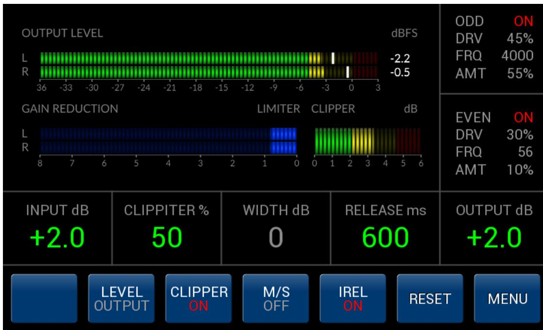
Most of the screen is occupied by the **OUTPUT LEVEL** meter (it can be switched to the input monitoring mode), the **GAIN REDUCTION** meter, that shows the amount of reduction applied to the signal by the VCA limiter, and **CLIPPER** meter showing how much of the signal amplitude have been “cut” by the clipping circuit (only if the Clipper is enabled).
