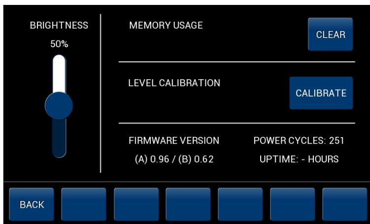
This screen allows you to adjust the **BRIGHTNESS** of the screen (touch and drag the virtual slider on the screen), check the firmware version of your unit, see the number of power cycles (how many times the unit was turned off and on), but also to **CLEAR** presets memory and perform the **CALIBRATION** procedure (it has to be done only once when you connect the
