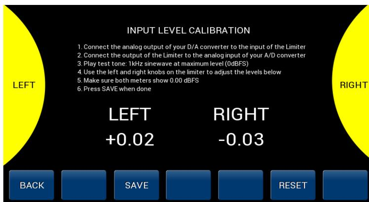
The mastering limiter is prepared to work straight from the box. In most cases the metering will be accurate and the limiter will behave perfectly. However if you would like to calibrate the 0dBFS reference with your D/A converter super precisely, we have added an option to do so.
