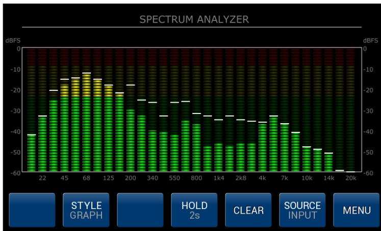
The spectrum analyzer window gives you a great, real-time insight into the current frequency content of the processed signal. By pressing the **STYLE** button you can choose two types of graphical representation to fulfill your needs. BARS style with 30 animated meters and peak hold functionality (you can personalize this feature by
